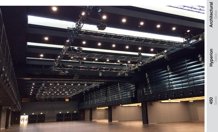
In the Performing Arts, the quick maintenance and reliability are fundamental: the HALLED guarantees both thanks to the remote location of the driver and power supply.
